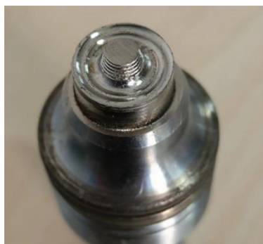
图 2-4 13 mm 轴肩搅拌头形状与搅拌头尺寸示意图 Fig. 2-4 13 mm shoulder stirring head shape and stirring head size diagram
