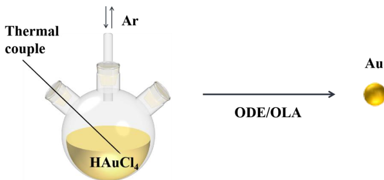
Fig. 2-2. Schematic diagram of gold particle synthesis
