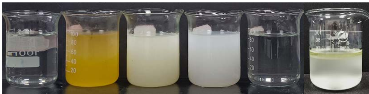
图 2-2.不同类型合成液的照片。从左至右依次为: 纯水、乙二醇、丙二醇、丁二醇、戊二醇、己二醇 Fig. 2-2 Photographs of synthetic solutions prepared with different types of organic solvents. From left to right: Pure water, ethylene glycol, 1,3-propanediol, 1,4-butanediol, 1,5-pentanediol, 1,6-hexanediol
