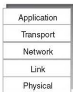
Figure 5.2 TCP/IP network model.
