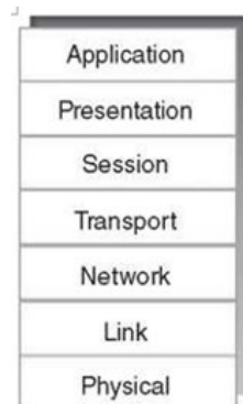
Figure 5.1 OSI layered network model.
